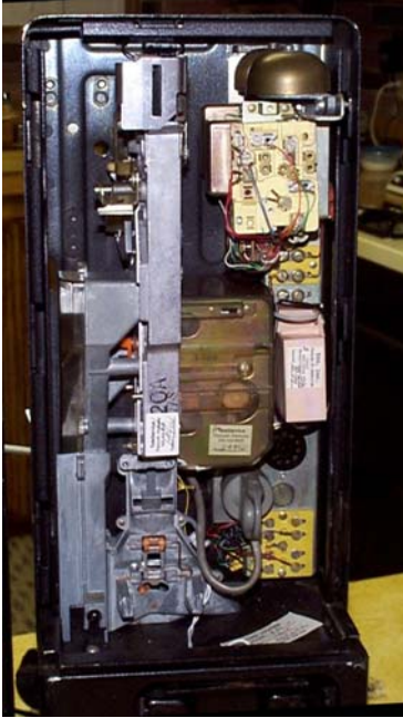
A Modern Single Slot – No Coin Relay
