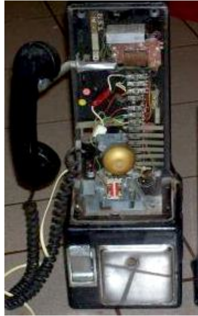
A 3 Slot – Bell in place of Coin Relay
