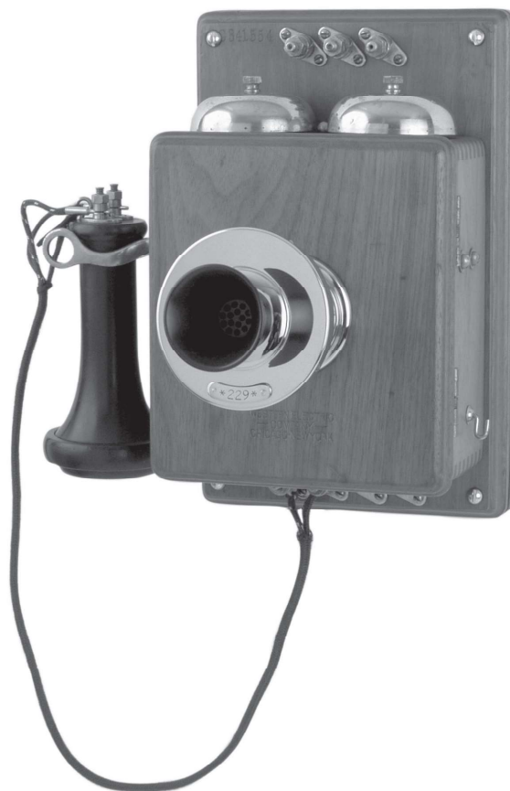
FIGURE 6.2 Western Electric's first wall phone with the booster circuit, ca. 1900. (Photo by Marketa Ebert.)
