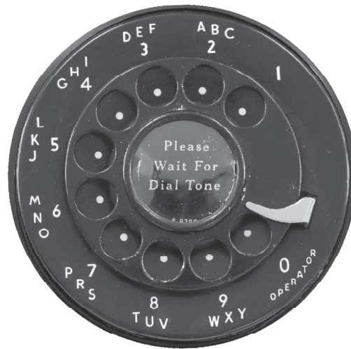
FIGURE 21.5 White aiming dots beneath the holes in a finger wheel.
