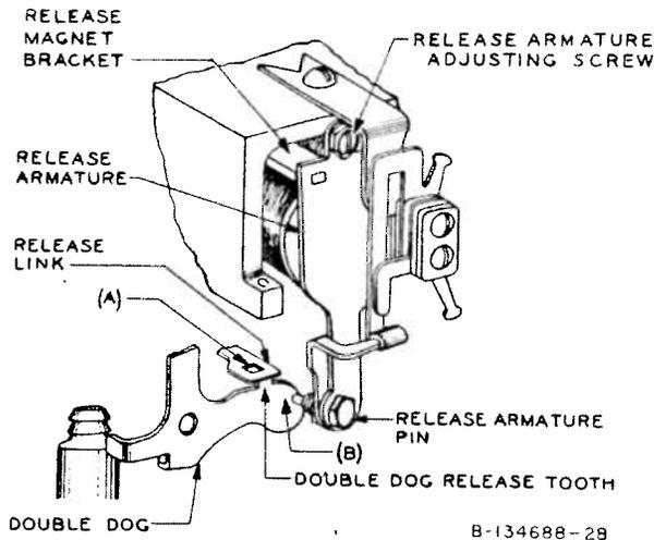
**Fig. 28—Release Magnet and Earlier Type Associated Parts**
