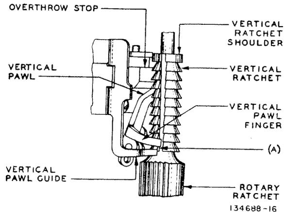
Fig. 16—Relation of Vertical Pawl to Vertical Ratchet
