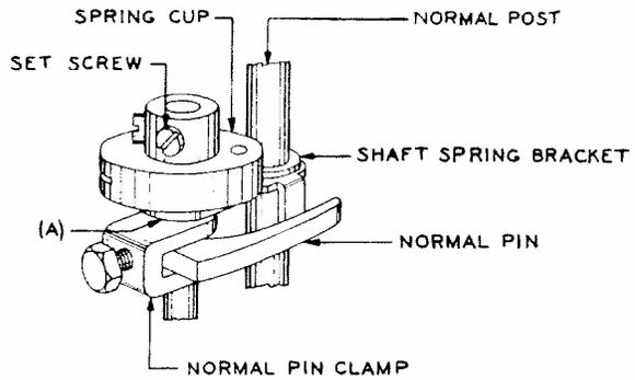
**Fig. 11—Spring Cup and Associated Parts**
