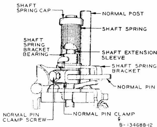
Fig. 12—Helical-Type Shaft Spring and Associated Parts
