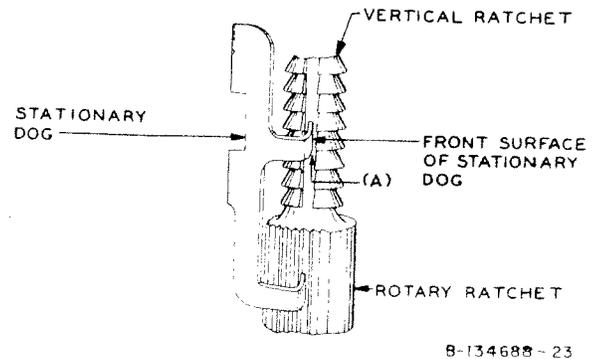
**Fig. 23—Horizontal Alignment of Stationary Dog**
