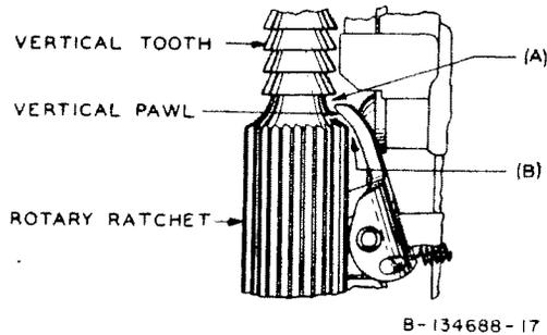
**Fig. 17—Clearance Between Vertical Pawl and Vertical Teeth**
