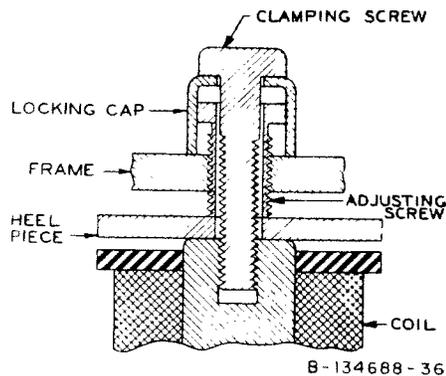
**Fig. 36—Vertical Magnet Clamping Screw and Associated Parts**
