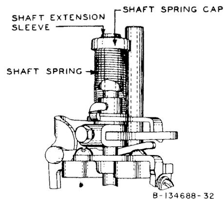
**Fig. 32—Helical-Type Shaft Spring**
