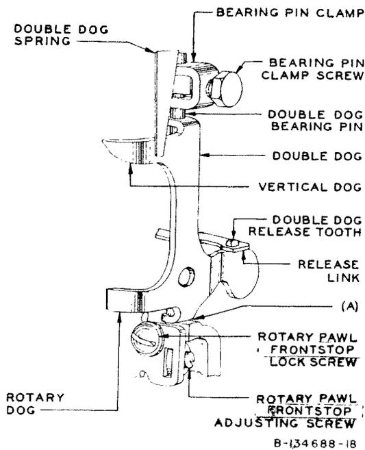
**Fig. 18—Double Dog and Associated Parts**
